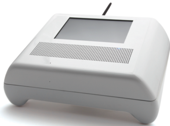
Figure 1: Highly reconfigurable portable software radio prototype implemented using open-source software and predominantly COTS hardware. The prototype provides dynamically configurable multi-channel and full-duplex communications in most frequency bands from 50 MHz to 2.9 GHz.
